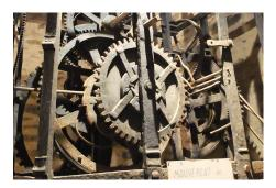
Although most clocks move at a perceptible speed, others can be very fast or very slow. For example, it is possible to build a clock that ticks once every millenium by linking together multiple axles with very large gear ratios.
